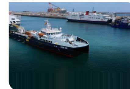
These vessels are an integral component of the logistics chain for offshore drilling rigs, platforms and other installations due to their speed, versatility and ability to carry up to 150 passengers at a time. These vessels offer a more environmentally sound, safe, cost-efficient, comfortable and flexible alternative to helicopter transportation of passengers.
